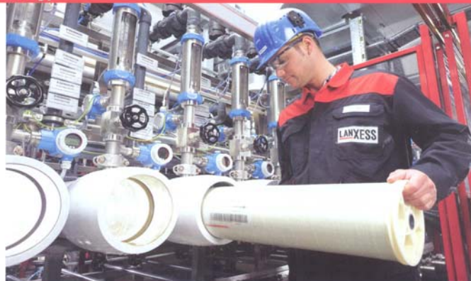
For quality assurance purposes each individual Lewabrane module is checked in an element tester at the LANXESS site in Bitterfeld Germany
