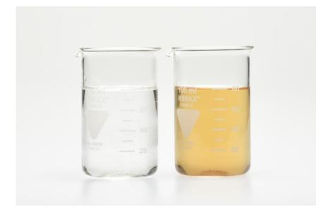
Ion exchange resins and membrane elements from LANXESS work hand in hand in power plants to turn surface water (right) into boiler feed water. In a lot of cases organic carbon (TOC) could be removed to a great extent. TOC is undesirable because of the formation of carbon dioxide or organic acids which favors corrosion in power plant operation. Photo: LANXESS AG
