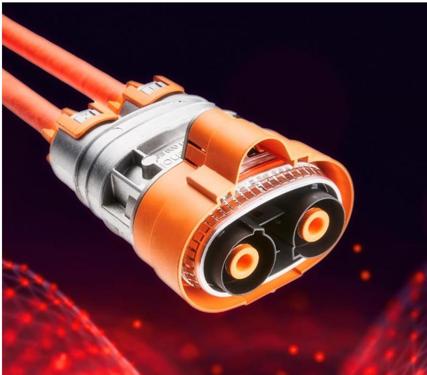
Connector made from Durethan BKV30FN04 for cable harnesses in electric models produced by a European-US automotive manufacturer. The halogen-free flame-retardant polyamide 6 can also be dyed in bright colors like orange (RAL 2003) and yellow and is characterized by its high strength and toughness.
